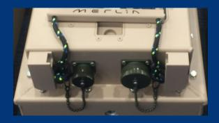
On the front of the PowerCentre there are two military connectors, one for AC input and one for DC output.
